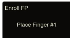
Place the finger on sensor scanner. Please follow the screen prompts to register the fingerprint.
